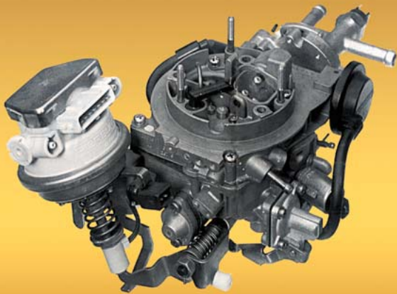
Carburetor with Electronic Idler control
